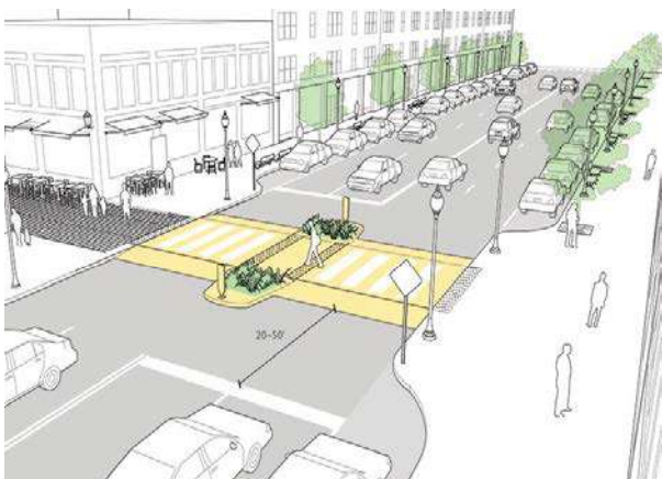
Midblock crossing where blocks may be too long for pedestrians to cross at intersections. The pedestrian refuge island allows for a safe place for pedestrians to stop so there is less conflict with on-coming traffic. Photo source: NACTO
